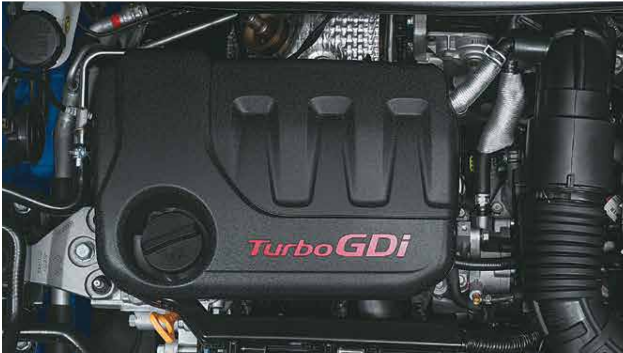
1.0 I Turbo GDi petrol engine with max. power of 88.3 kW (120 PS) / 6 000 r/min
